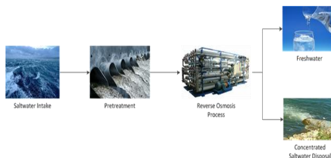
Fig. 1. Reverse osmosis process stages
