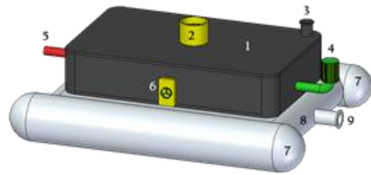
Fig. 6. Offshore reverse osmosis unit
